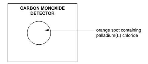
The orange spot turns black if there is a high concentration of carbon monoxide in the air.
